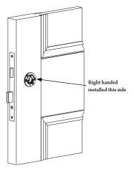
Insert the fixing bolts through the horizontal holes of the rota-bearing sprung rose from one side, and the fixing nuts from the other side, then tighten together. The bolts may need to be shortened depending on the thickness of the door at one of the cut-off points along the length of the bolt.
