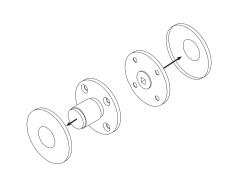
**2.** Assemble thumb turn with the square bar and screws provided
